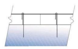
Cross section of installed Geocell
